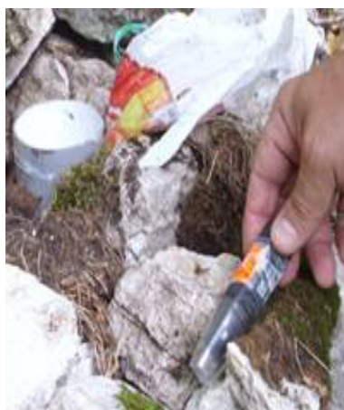
Fig. 4.a. Data-logger and upper opening of the poll
