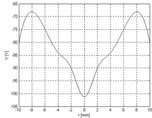
**Figure 3.** The radial distribution of the electric potential for  $z=6$  mm
