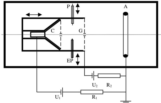
*Figure 1. The schema of the experimental device: C–cathode; G–control grid; A–anode; P–simple probe; EP–emissive probe;  $U_1$ ,  $U_2$ –power sources in CC.*
