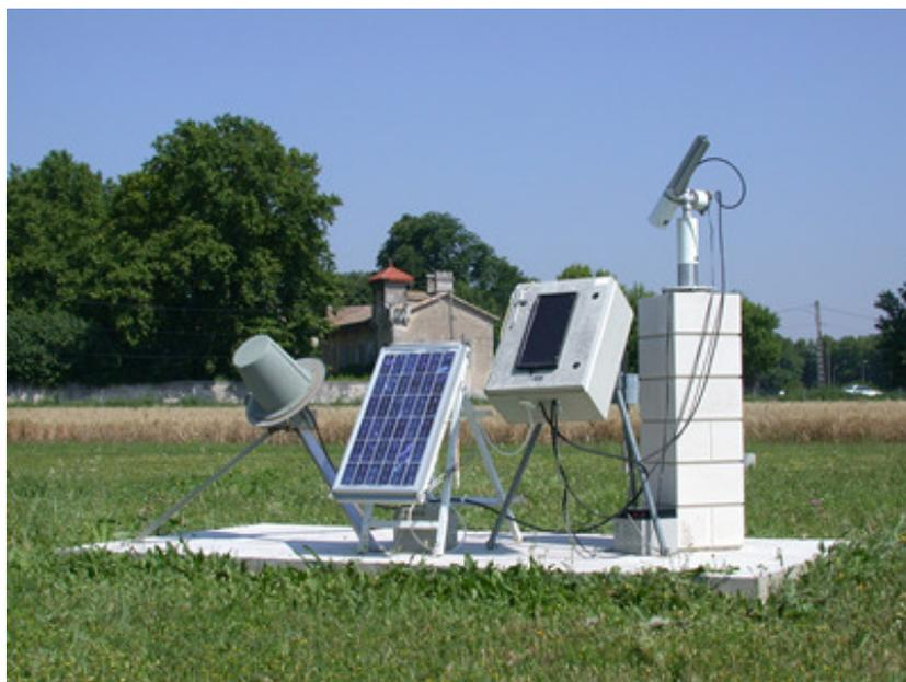
*Figure 9. Standard operational CIMEL platform used by AERONET station.*
