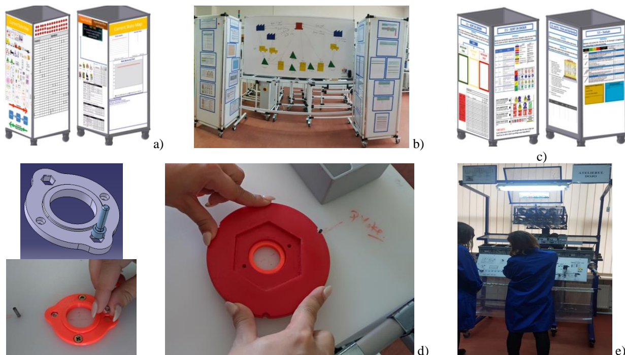
Figura 4. Platforme de experimentare Lean manufacturing: a) VSM; b) Lean corner; c) 5S; d) Poka-Yoke; e) DOJO
