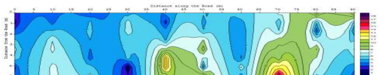
Figure 7. Distribution of frequency dependence magnetic susceptibility along selected road profile in Asokoro district
