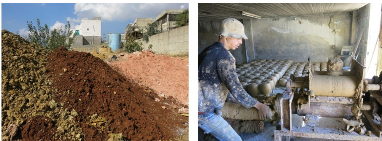
Fig. 11 Raw materials: yellow and red clay sediments and sand (left image); wedging the clay with a pug mill (right image). At this stage the salt is added to the clay material (photographs by V. Roux)
