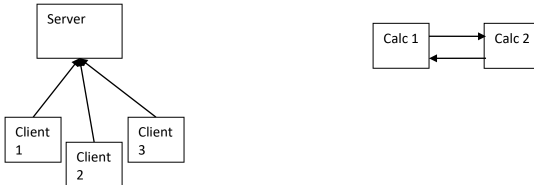
Retea centralizata server-client si retea descentralizata peer-to-peer.
